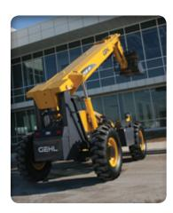
**SELF LEVELING** is a standard feature that automatically levels the forks or attachment as the boom is raised. This eliminates the need for manual adjustments.
