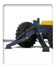
**OUTRIGGERS** increase stability and add to the lift capacity. Optional on the RS6-42, RS8-42, RS8-44, RS10-44 and RS12-42; standard on the RS10-55.
