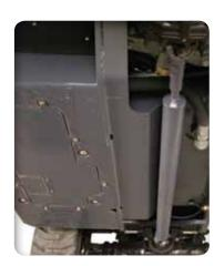
SERVICEABILITY is simple with a large, hinged hood on the side of the machine that lifts out of the way. A hinged door in the belly pan grants access to the oil drain.
