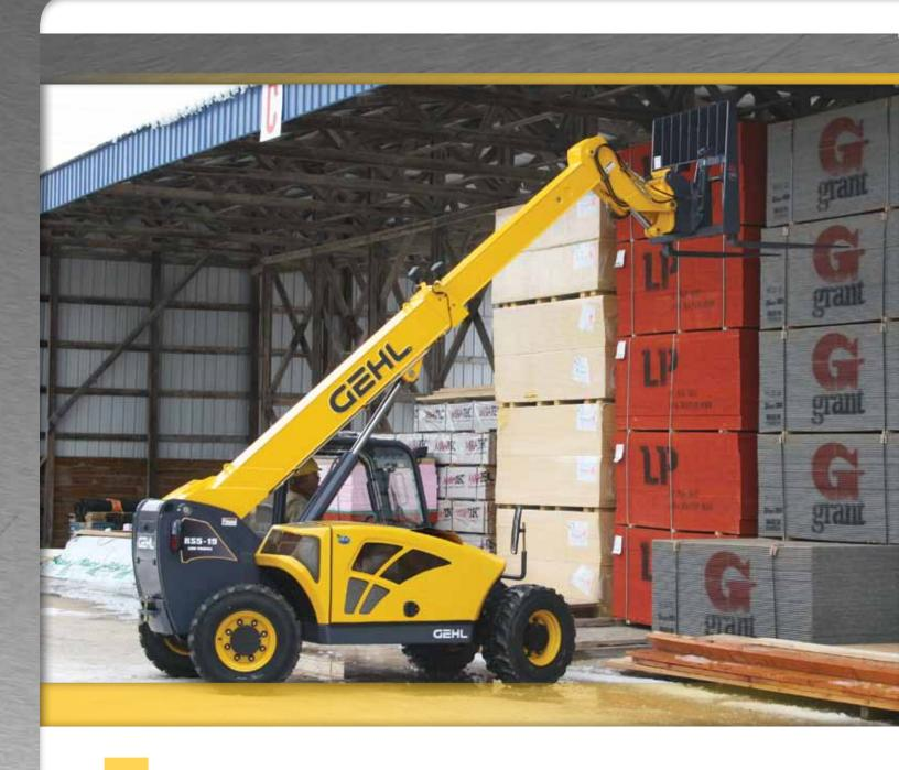
Size does matter . . . especially when working on confined jobsites. Standing only 6'4" tall with a turning radius of only 11 feet, this little giant makes working in confined spaces easy. With a lift height up to 19'1" and a maximum load capacity of 5,500 pounds, the RS5-19 creates big results, maximizing your investment.
