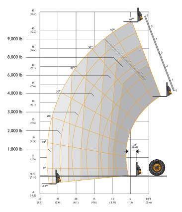
This load chart is for the rated capacity of the machine with 66" wide standard carriage and 48" pallet forks. Use only JCB approved attachments and check the relevant load chart for the machine model. If in doubt, consult your dealer.
