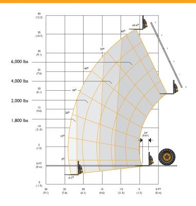
This load chart is for the rated capacity of the machine with 66" wide standard carriage and 48" pallet forks. Use only JCB approved attachments and check the relevant load chart for the machine model. If in doubt, consult your dealer.
