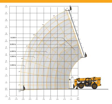
These load charts are for the rated capacity of the machine with 66" wide standard carriage and 48" pallet forks. Use only JCB approved attachments and check the relevant load chart for the machine model.
