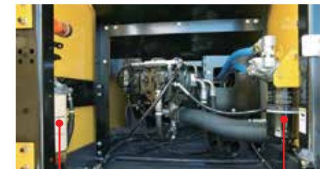
Fuel Filter (with built-in water separator)
